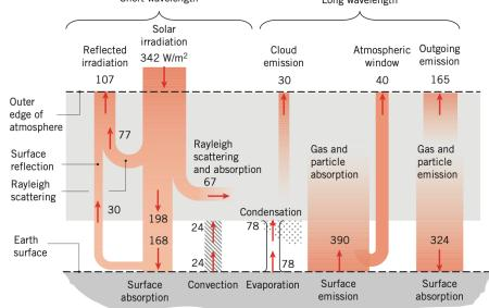
Figure 1. Breakdown of Atmospherical Energy Balance for Moderate Temperature and **Cloudy Conditions**
