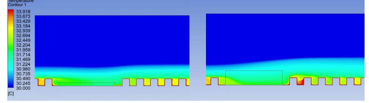
Figure 7. Temperature Contour plots of L10 D0p8 H0p05 (left) and L2p5 D0p8 H0p2 (right)
