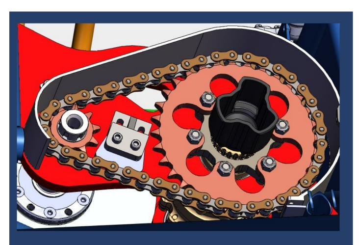
Current Design of Sprocket and Chain System with a tensioner by CUFR Team
