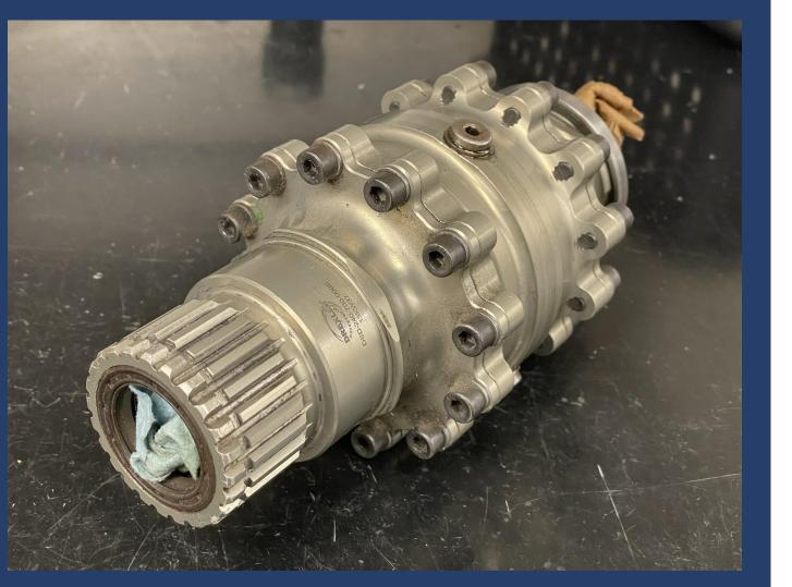
Differential Used In the Drivetrain System
