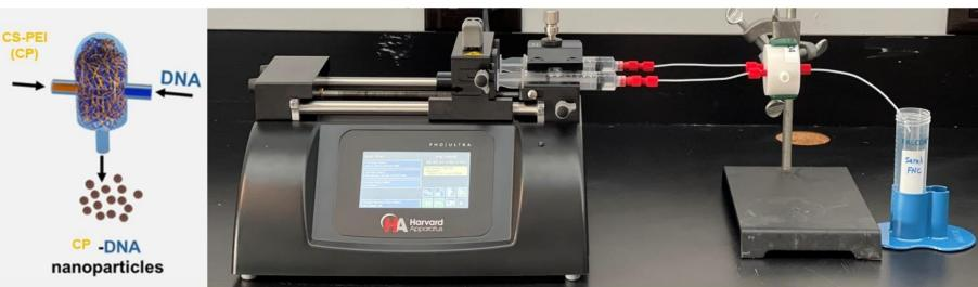
Figure 1: FNC apparatus used to create the NPs. The components flow from syringes into the mixing chamber, where they electrostatically complex in the turbulent flow before exiting into the test tube.
