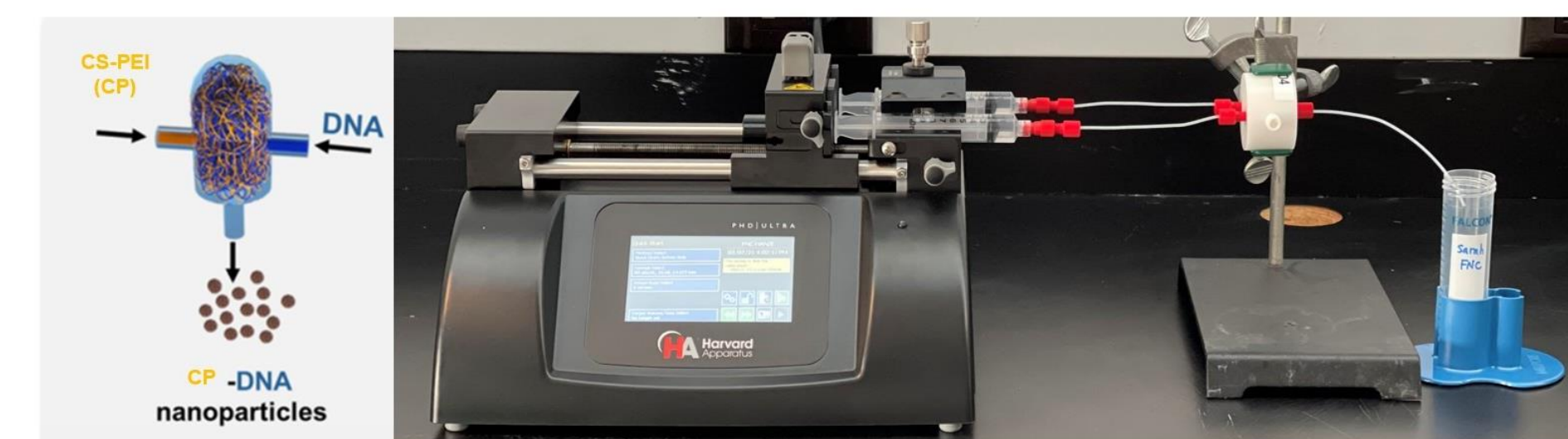
Figure 1: FNC apparatus used to create the NPs. The components flow from syringes into the mixing chamber, where they electrostatically complex in the turbulent flow before exiting into the test tube.
