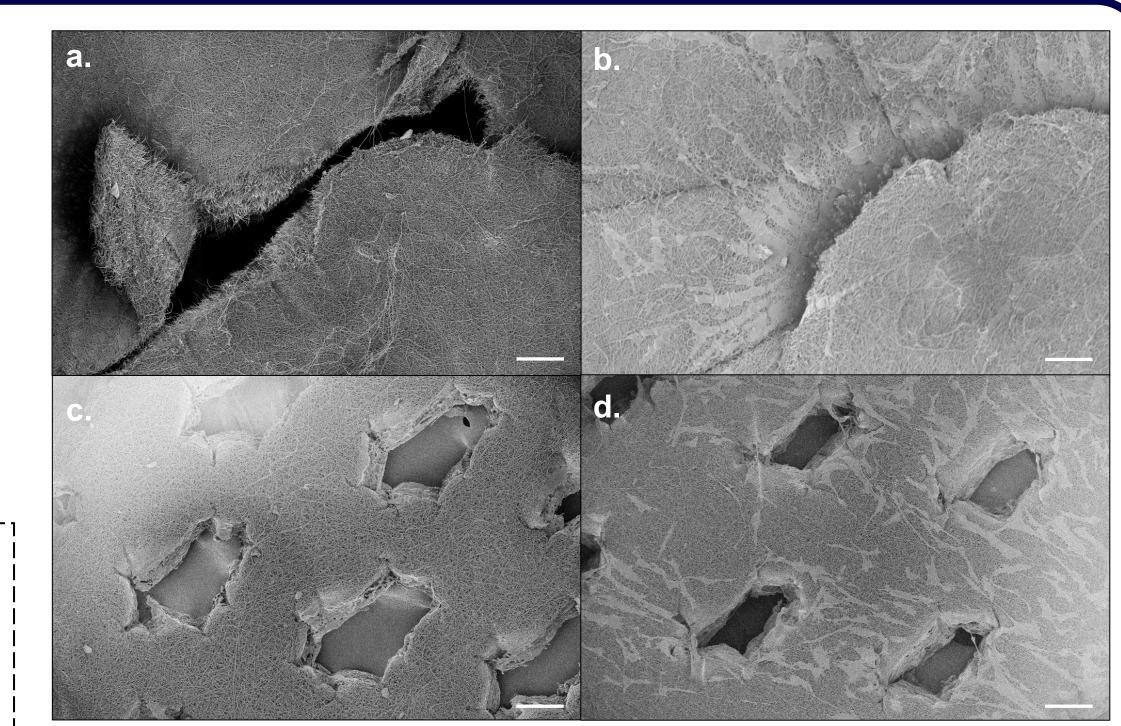
Fig. 3: SEM imaging of perforations pre- and post-cell culture. a/b. 18G hypodermic needle. *c/d.* Laser cut (200 μm diameter). Scale: 100 μm.
