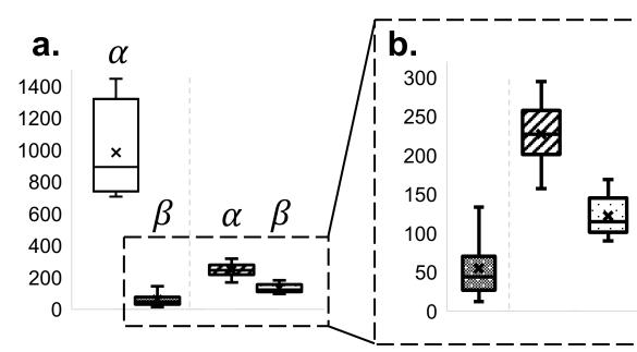
Fig. 4: a. Range of perforation sizes in µm; left: 26G, right: laser cut  $(\alpha = major axis, \beta = minor axis).$ **b**. Zoomed-in view of boxed region.
