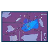
Figure 2. hBN, MoTe<sub>2</sub> stack Figure 3. Post etch/deposition
