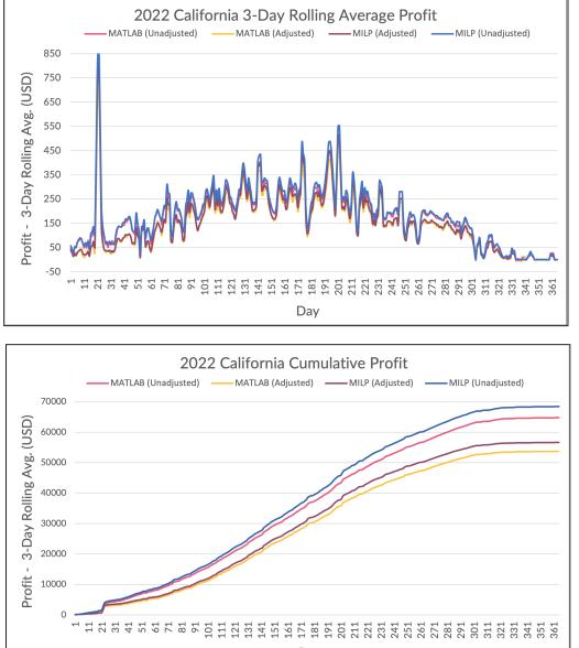
Profit vs. Execution Time: When comparing simulations with similar CO<sub>2</sub> adjustments (adjusted or unadjusted), MATLAB is up to 745 times faster with a <5% difference in profit from the benchmark, making it useful for generating electricity demand bids.
