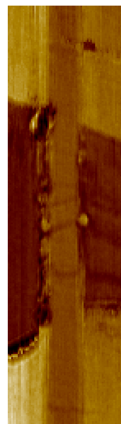
AFM images of etched WSe 2 with increasing frequency
