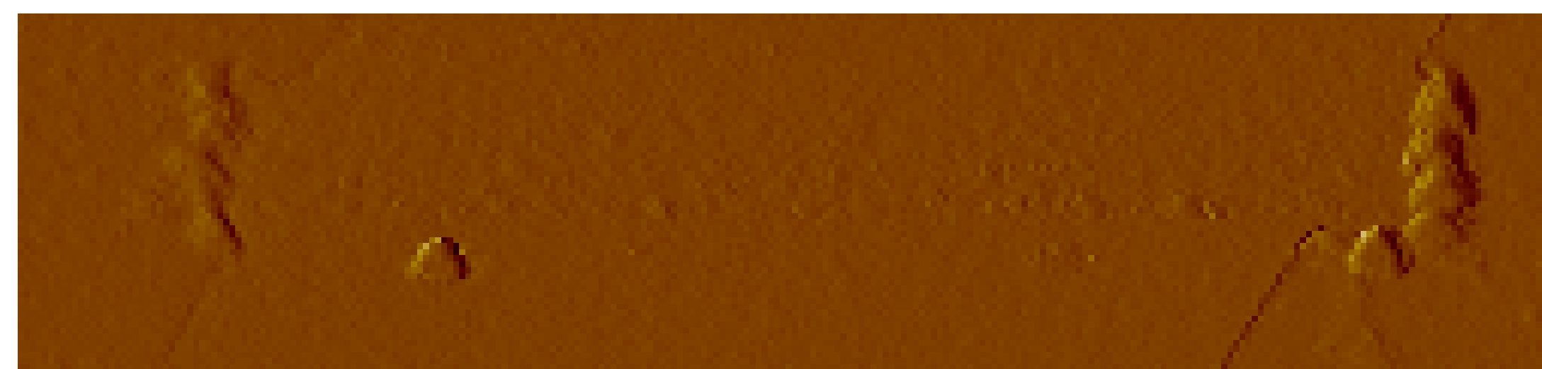
AFM images of etched WSe 2 with varying tip velocities
